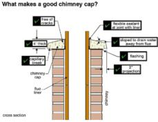
The chimney should be tall enough that it is not affected by wind swirling around other building components. It should be two feet higher than anything within ten feet of it.
