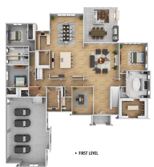
85'-2" x 100'-4" FOOTPRINT 10' MINIMUM to 17'-2" CEILING HEIGHT STEPPED/VAULTED PER PLAN
